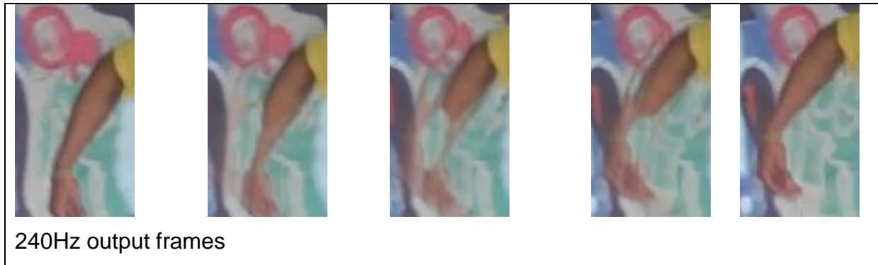
Figure 2 - Illustration of interpolation from 60Hz to 240Hz
