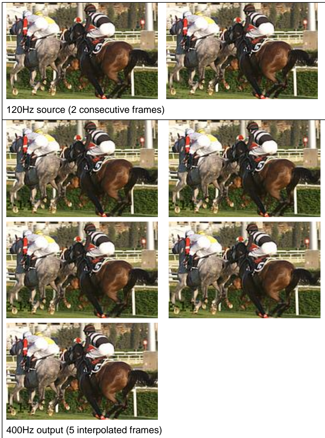
Figure 5 - Illustration of motion compensated interpolation from 120Hz to 400Hz
