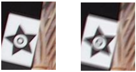
Figure 4 : Comparison of two deinterlacers (a) Preserving resolution (left) (b) Loss of picture detail (right)
