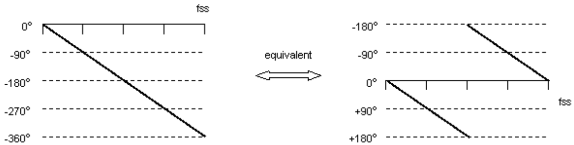
Figure 31: Phase response of the example time-shifter.
