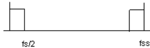
Figure 13: The ideal filter response for interpolation.
